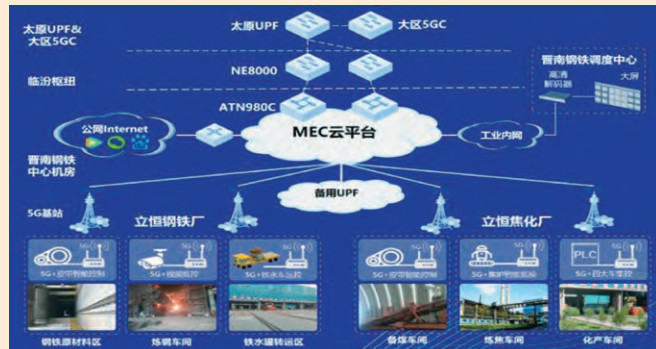
Jinnan Steel's 5G + Industrial Internet Architecture
